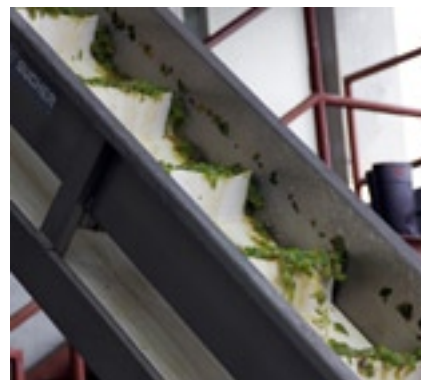
Crushed grapes and juice move up a conveyor belt to the press.
